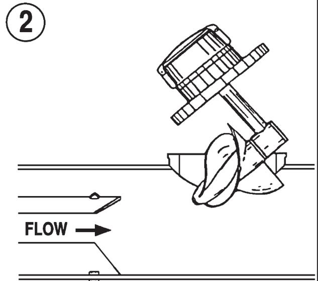
2. Tilt the meter head assembly forward allowing the propeller to move through the opening.
