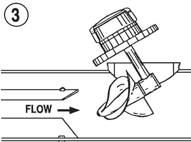
3. Slide the assembly forward and down. The propeller may have to be rotated in order to fit through the saddle opening.
