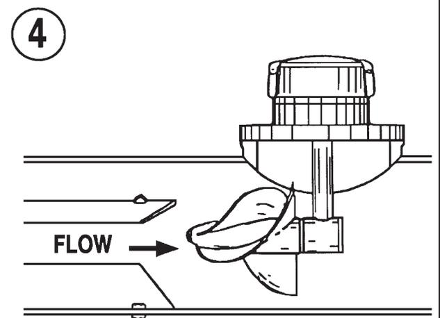
4. Allow the meter head assembly to come to rest on the saddle. Install bolts and tighten to proper torque.
