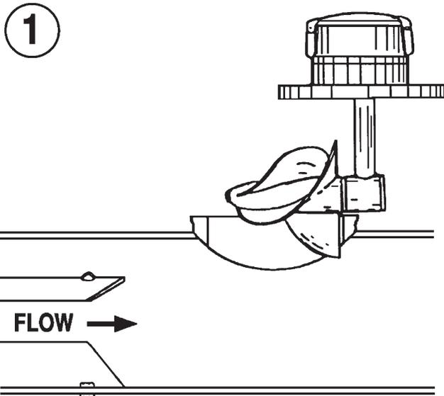
1. Set meter assembly on saddle as shown with one propeller blade pointing down. Propeller should point opposite the direction of flow.
