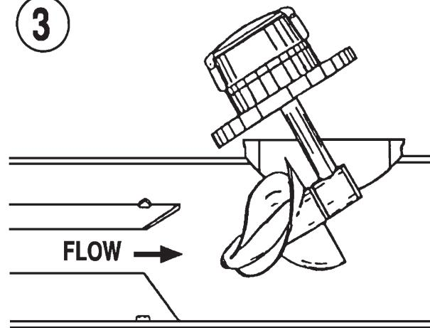
3. Slide the assembly forward and down. The propeller may have to be rotated in order to fit through the saddle opening.
