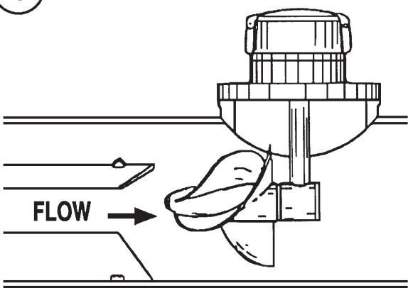
4. Allow the meter head assembly to come to rest on the saddle. Install bolts and tighten to proper torque.
