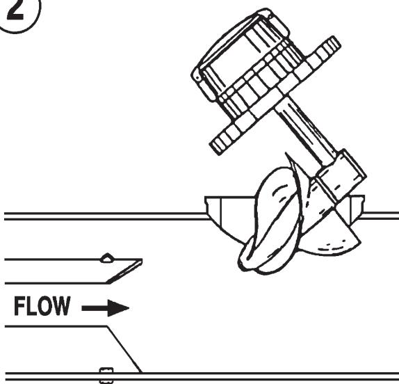
2. Tilt the meter head assembly forward allowing the propeller to move through the opening.
