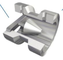
The Wafer-Cone is available in line sizes from 1 to 6 inches and can be oil or gas flow calibrated. Featuring a removable cone and flangeless design, cones with different beta ratios can be easily exchanged to accommodate changing flow conditions without the need for recalibration.
