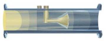
As the flow approaches the cone, the flow profile "flattens" toward the shape of a well developed profile—even in extreme flow conditions.
