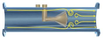
The V-Cone's contour-shaped cone directs the flow towards the outside wall away from the cone. As a result, the beta edge is not subject to wear by particle laden fluids and remains unchanged. Therefore, V-Cones rarely, if ever, require recalibration or replacement.
