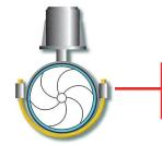
The positioning of the impeller directly in the flow stream assures full-flow measurement and greater accuracy.
