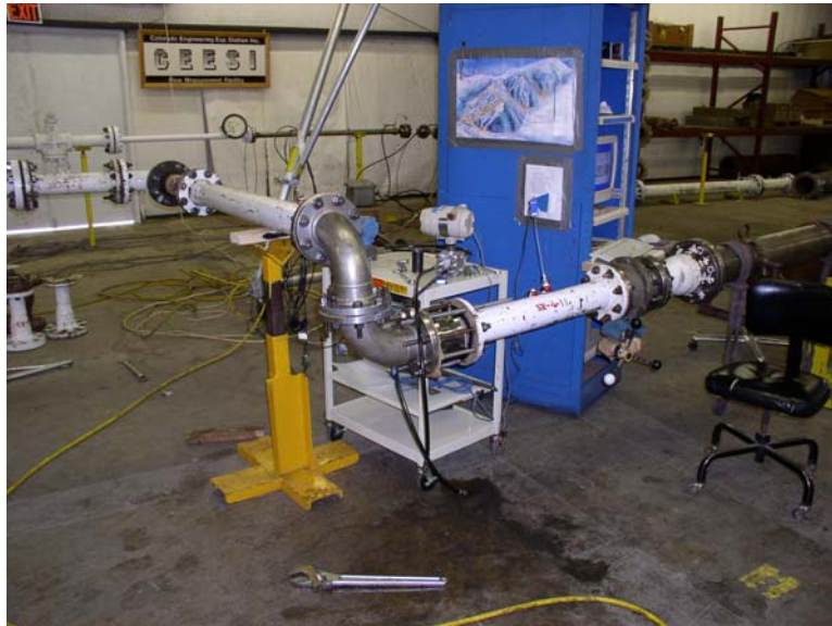
Fig. 5 Out-of-Plane Elbows Test Setup
