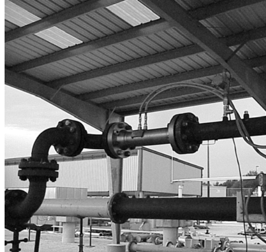
Figure A-8. Non-Standard Test 2: Installation of 4-inch Test Meter Immediately Downstream of Double 90° Out-of-Plane Long-Radius Elbows. The entire installation is shown at left and the V-Cone meter up-close is shown at right.
